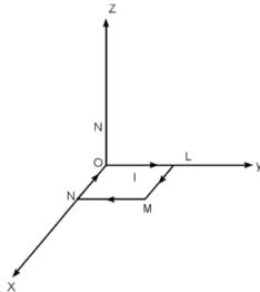
A given rectangular coil OLMN of area A, carrying a given current I, is placed in a uniform magnetic field  $\vec{B} = B \hat{k}$ , in the orientation shown here, What is the magnitude of torque experienced by this coil?
